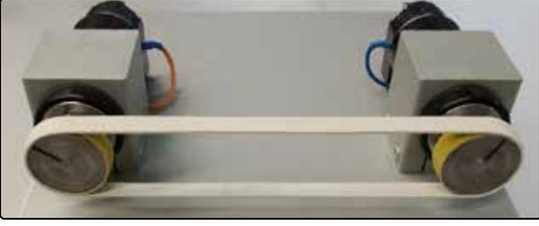
Fig. 3. Illustrative setup with two DC motors and elastic connection.
