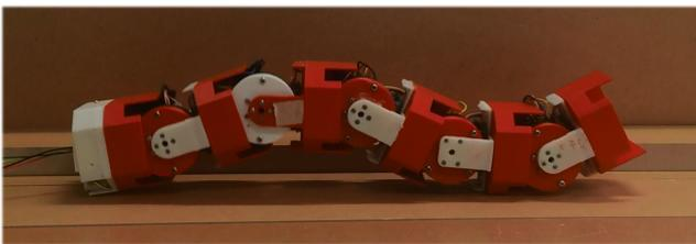
**Figure 1:** Rectilinear locomotion of a modular snake robot.
